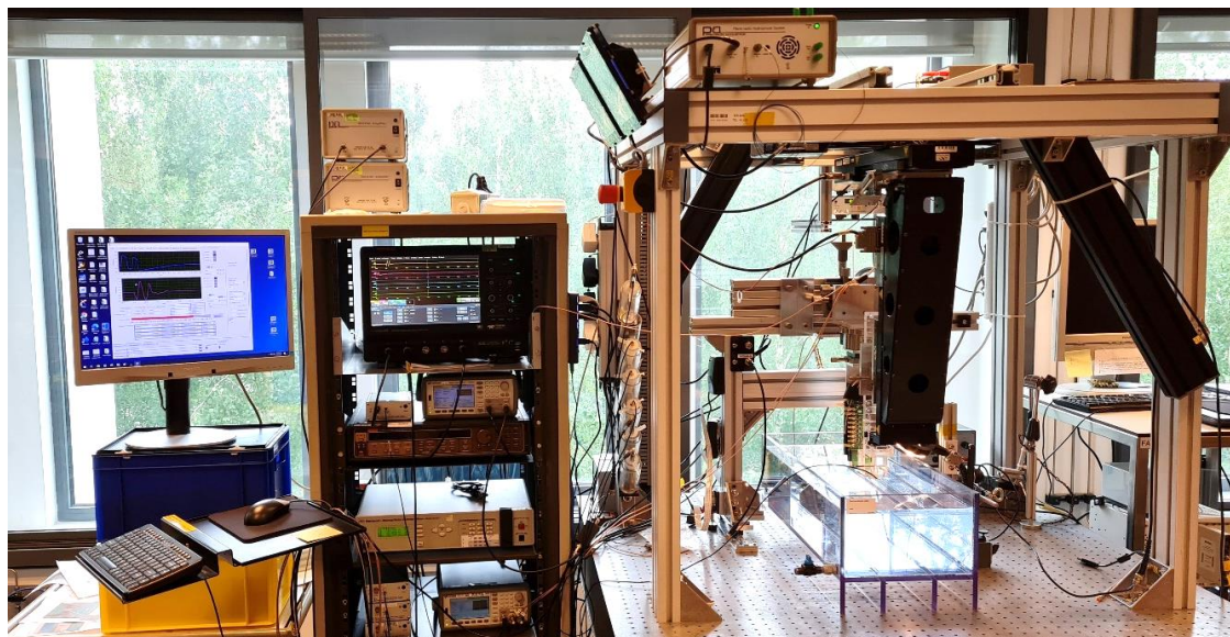
Figure 15 The set-up used for acoustic measurements (overview).
